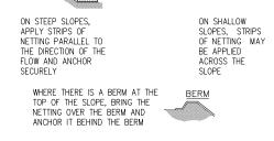
TO PROVIDE IMMEDIATE PROTECTION TO EXPOSED SOILS. DURING THE PERIOD OF SHORT CONSTRUCTION DELAYS
